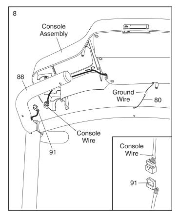
Set the console assembly on the Left and Right Handrails (87, 88). Be careful not to pinch any wires. Insert the excess Upright Wire (91) into the Right Handrail, and insert the Console Ground Wire (80) into the console assembly.
